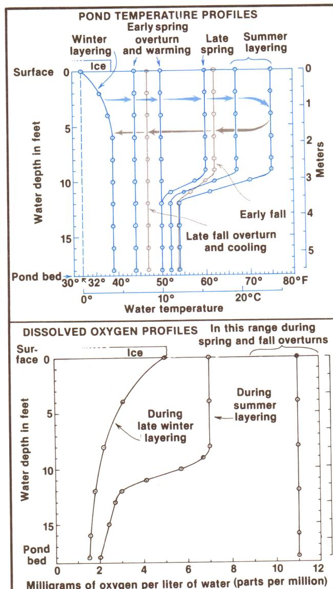
Dissolved oxygen at different depths in the same pond, as affected by the wind mixing and thermal/density layering shown in the figure on page 20.
