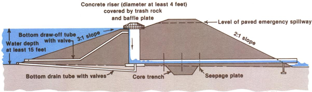
Two common types of outlet structures for dams that form fish ponds. Riser-and-stoplog construction is the simplest design that allows controlled bottom draw-off. A drop-inlet spillway can accommodate greater variation of flow. It is needed where run-off from large land area supplies the pond and where sudden high water is expected.
