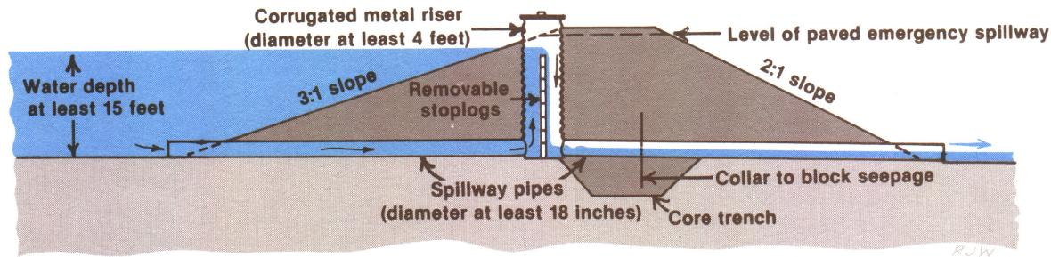
**SURFACE OVERFLOW DAM — WITH DROP INLET SPILLWAY AND OPTIONAL BOTTOM DRAW TUBE**
