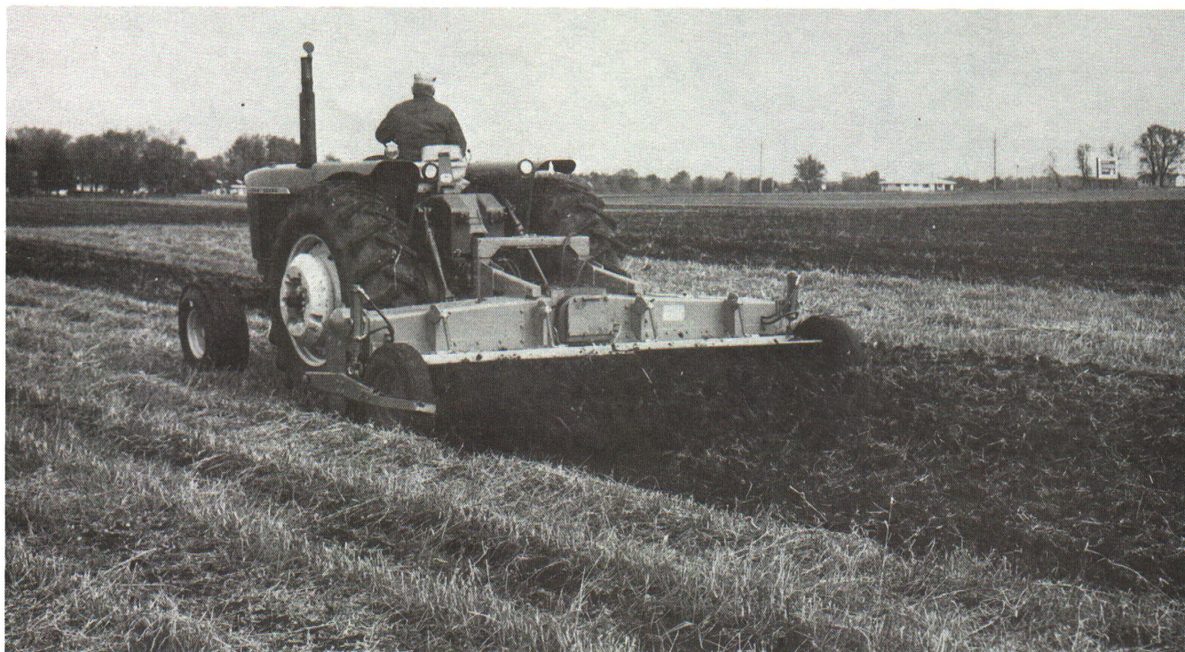
Figure 10 —Rotary-type plows are used most extensively on specialty farms, although there is increased interest on others because it can produce clod-free soils. It is especially well adapted for the incorporation of manure and compost materials. Tillage depth is limited, and power requirements are generally higher than with other implements. Where rotary type plows are used as a once-over tool, power requirements will be lower than in those systems that involve secondary or supplemental treatments.
