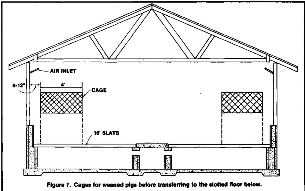
Figure 7. Cages for weaned pigs before transferring to the slotted floor below.
