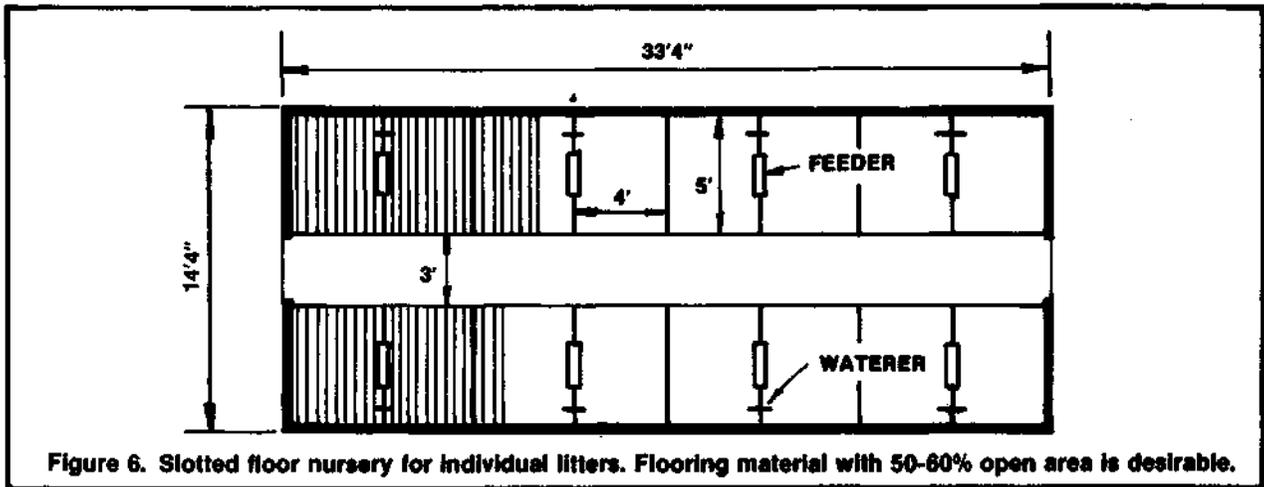
Figure 6. Slotted floor nursery for individual litters. Flooring material with 50-60% open area is desirable.
