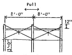
Fig. 2. Wood line pull brace. Use every 40 rods in long fences.
