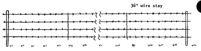
Fig. 4. Suspension fence construction. Posts up to 100 ft. apart. Twisted wire stays 10 to 15 ft. apart.
