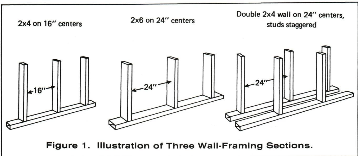
16 in. or 24 in. centers is becoming more popular in an attempt to approach "superinsulation" while still using more or less standard framing techniques. Finally, double-wall framing is sometimes used, with potential R values of 40 and more (see Figure 1). Other, more exotic, superinsulation techniques have been successful, but generally result in high labor or material costs and questionable return on investment.
