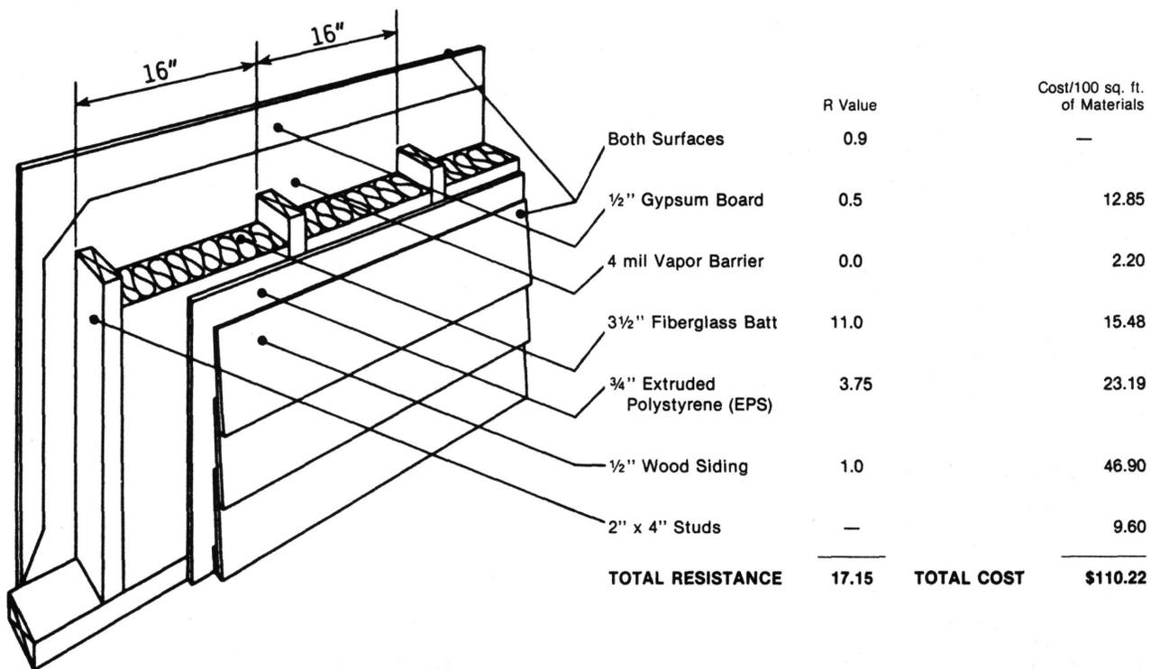
**Figure 3. Fiberboard Replaced with Extruded Polystyrene (EPS).**
