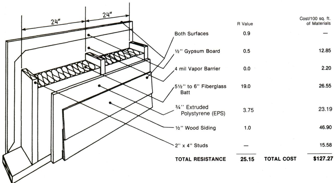
**Figure 4. A 2 x 6 Framing Technique with EPS.**
