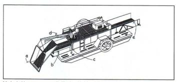
Mechanical harvesters are not all alike, but this 36' paddle-wheel driven unit with a front mounted aquatic plant-cutter illustrates some of the most important inspection points: a) front cutting table, b) front conveyor belts, c) frame members, d) hydraulics e) rear storage conveyor
