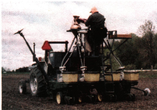
In 1990 this 4 row vacuum planter was purchased for the trials. It has been up dated in 1994, 2001 and 2003 to keep it current with new technology.
