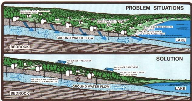
Generally soils that are a mixture of sand and clay work best if not overloaded. Although soil and water table factors are very important to the efficient operation of the septic tank/drain field system, the ideal soil-water table situation can become saturated, ineffective
