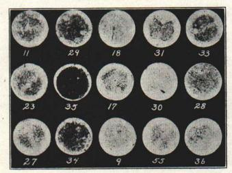
Each of these discs show the dirt contained in one pint of milk. The milk samples were obtained from Michigan farms in a whole milk area. The clean discs in the upper cut show clean milk production under conditions as explained in this bulletin.
