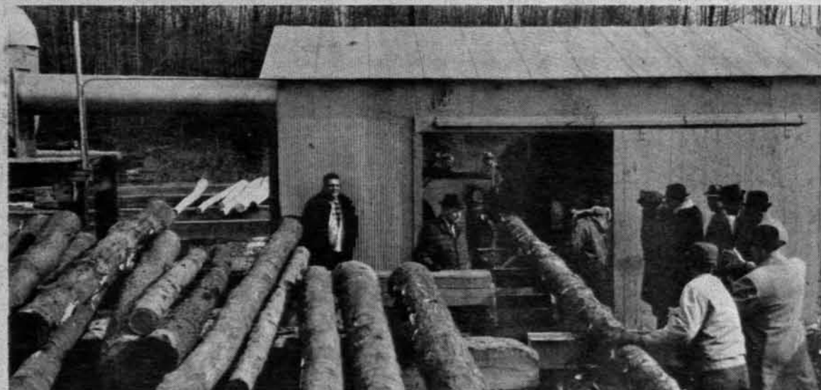
TREATED POLES — at the John A. Biewer Company plant in St. Clair begin as trimmed trees direct from the forest. They end as smoothly barked and pressure-treated timbers, ready for use in Farm Bureau pole buildings. A "trainload" at a time of the peeled poles is shunted into a cavernous cooker which pressure treats the wood to assure permanence. Fence posts and some forms of lumber are also treated.
