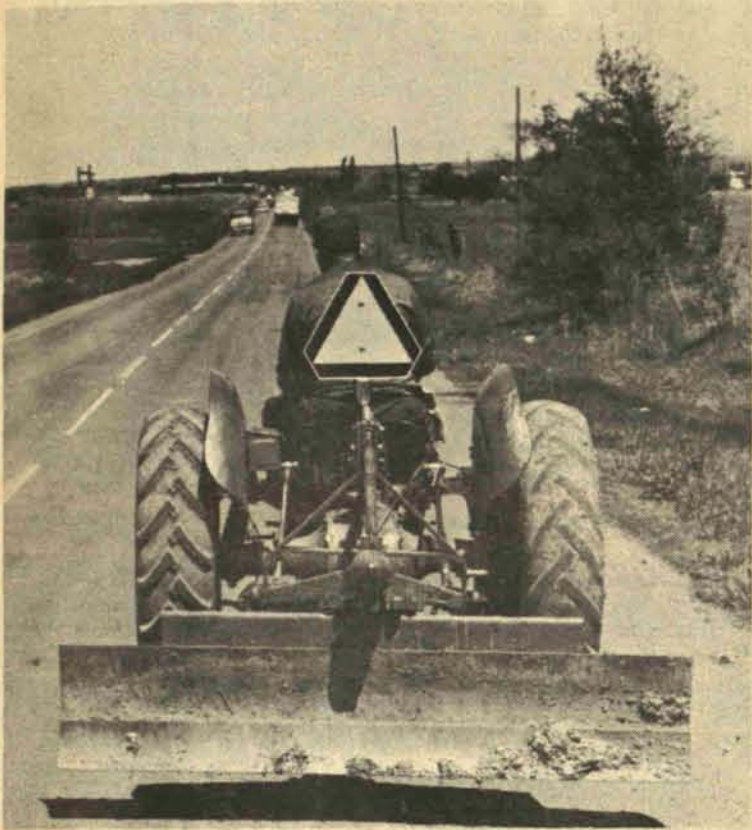
SLOW-MOVING VEHICLE — farm safety emblem, appears with growing frequency on Michigan farm machinery. Especially designed to eliminate rear-end highway collisions, the bright emblem includes a red reflective border around a triangle of fluorescent orange.
