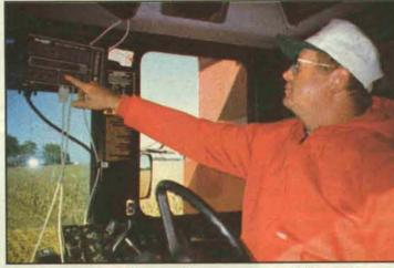
John Woodhouse checks the yield monitor mounted in the cab of his combine. Woodhouse is using precision agriculture technologies to build a database of detailed, site-specific information about his crop production system.
