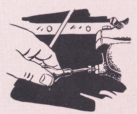
Fig. 11 Adjusting load valve.
