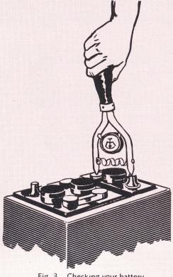
Fig. 3 Checking your battery with a voltmeter.
