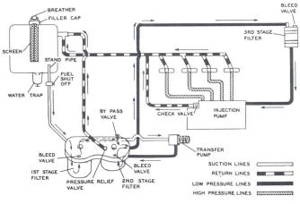
Fig. 13 Parts of a diesel fuel system.
