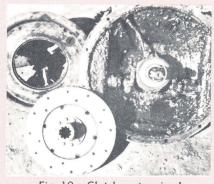
Fig. 10 Clutch parts ruined by over-greasing.
