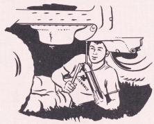
Fig. 11 Greasing a clutch pilot bearing.
