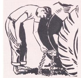
Fig. 18 Ground your tractor when doing belt work.
