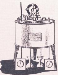
Fig. 6 A viscosity tester.
