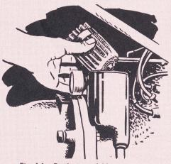
Fig. 14 Replacing oil filter element.
