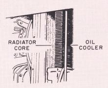
Fig. 3 On some tractors, the hydraulic system oil is cooled by air drawn through the radiator.
