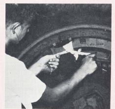
Fig. 11 Check slippage by tying a cloth to a spoke and counting off 30 revolutions.
