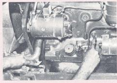
Fig. 18 Two places to drain the cooling system.
