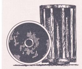
Fig. 17 Plugged filter and screen.
