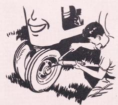
Fig. 13 Greasing a front wheel.
