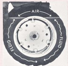
Fig. 8 Add calcium chloride and water to rear tires for additional weight.
