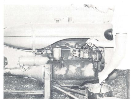
Fig. 17 Cleaning up ignition parts.
