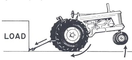
Fig. 10 The load tries to raise the front end of the tractor.
