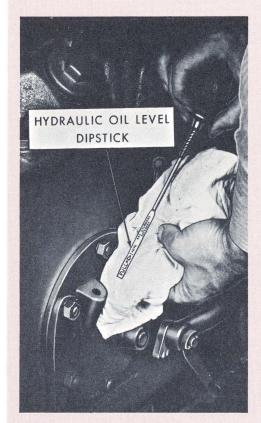
Fig. 25 Maintain the hydraulic system oil level.
