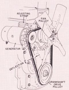
Fig. 13 Keep the fan belt properly adjusted.
