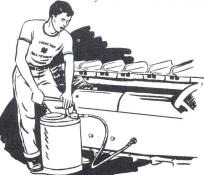
Fig. 14 Greasing track rollers.
