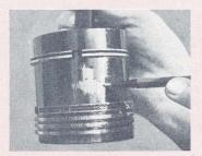
Fig. 8 Test piston shows varnish - non-additive motor oil.
