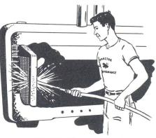
Fig. 15 Washing out the radiator.
