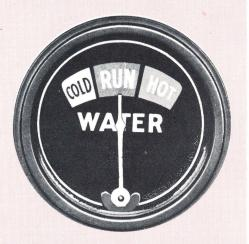
Fig. 2 A cooling system temperature gauge.
