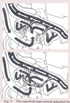
ig. 5 The manifold heat control adjusted for warm weather (top) and cold weather (bottom).
