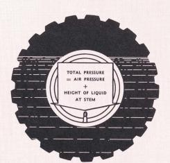
Fig. 2 Valve stem should be at the bottom when testing pressure of liquid-filled tire.
