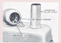
Fig. 12 Don't forget to clean the crankcase breather.
