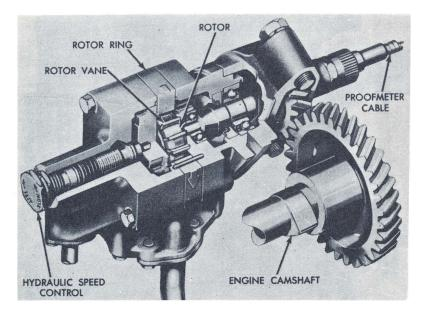
Fig. 27 Hydraulic pump cut apart to show construction.
