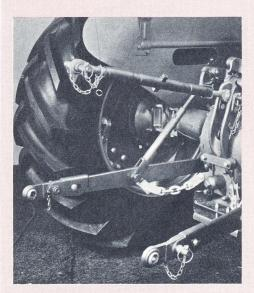
Fig. 26 A three-point, hydraulically controlled implement hitch.
