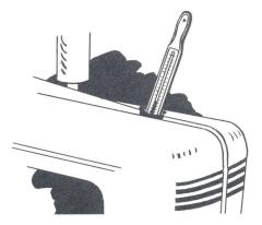
Fig. 9 Measuring radiator temperature.
