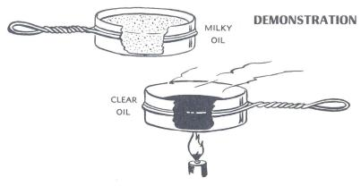
Fig. 20 Heating milky oil drives off water and makes the oil clear
