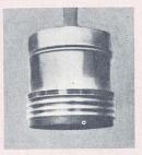
Fig. 9 Clean test pistonadditive motor oil.
