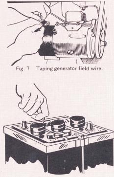
Fig. 8 Tightening the battery.
