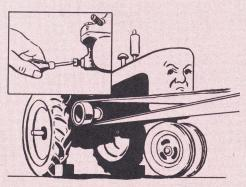
Fig. 12 Adjust the load valve when doing belt work.
