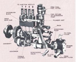
Fig. 2 A diesel engine fuel system.
