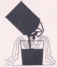
Fig. 18 Fuel vapors are heavier than air.
