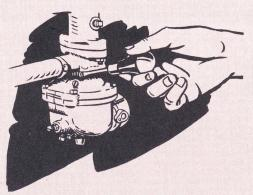
Fig. 9 Adjusting the idling speed.
