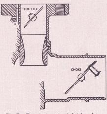
Fig. 7 The choke cuts air intake when starting a cold engine.
