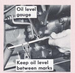
Fig. 2 Check the crankcase oil level every time you use the tractor.
