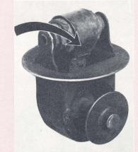
Fig. 6 A metal strip thermostat that has been ruined by scale.
