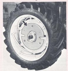
Fig. 9 Wheel weights can also be used to add weight to the rear wheels.
