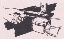
Fig. 10 Adjusting idling mixture.
