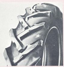
Fig. 15 Irregular wear caused by operating the tire at low pressure on a hard road surface.
