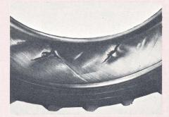
Fig. 16 Sidewall buckling due to constant use at too low a pressure.
