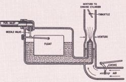
Fig. 4 Here is how a carburetor works.
