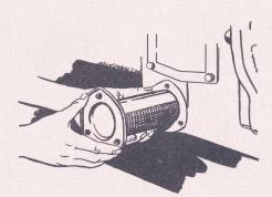
Fig. 18 Removing oil pump intake screen for cleaning.
