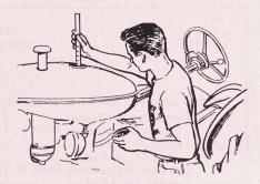
Fig. 4 A measuring stick makes it easy to tell how much fuel remains in the tank.
