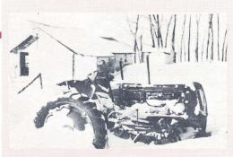
Fig. 16 After your tractor has been stand ing idle — look for water and dirt settling in crankcase.
