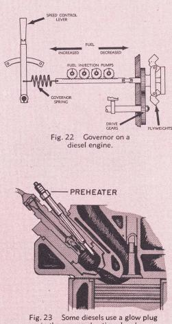
in the pre-combustion chamber for quicker starting.
