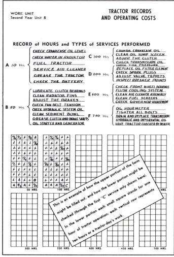
Fig. 2 A positive reminder of service required at regular intervals.
