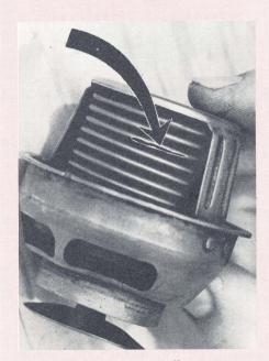
Fig. 7 A cracked bellows-type thermostat won't close.
