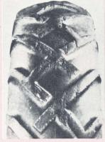
Fig. 7 Excessive slippage causes tread wear.
