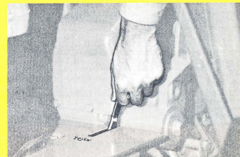
Fig. 26 Lever for disengaging transmission gears so tractor can be towed.
