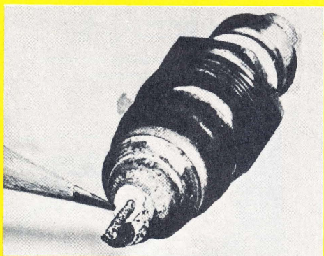
Fig. 21 Broken spark plug porcelain.
