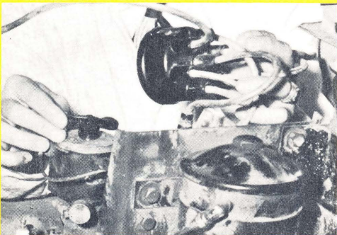
Fig. 10 Checking direction in which rotor turns.
