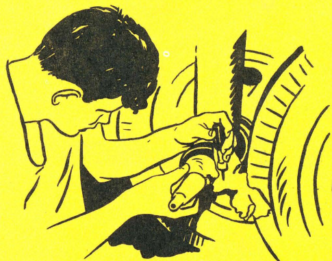
Fig. 18 Forcing grease into a bearing, using a cloth and a screw driver.
