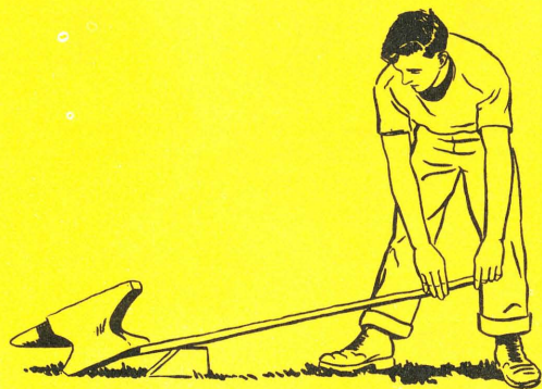
Fig. 2 Gears are like a long lever.
