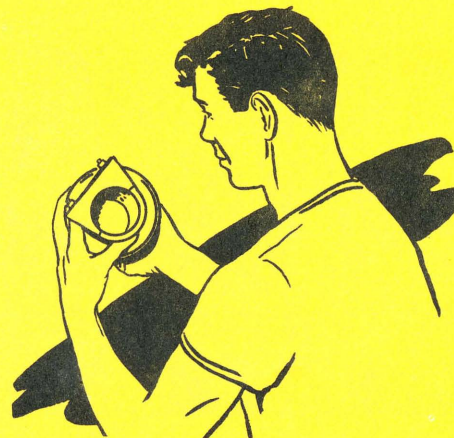
Fig. 20 Check the muffler for restrictions, dirt, etc.
