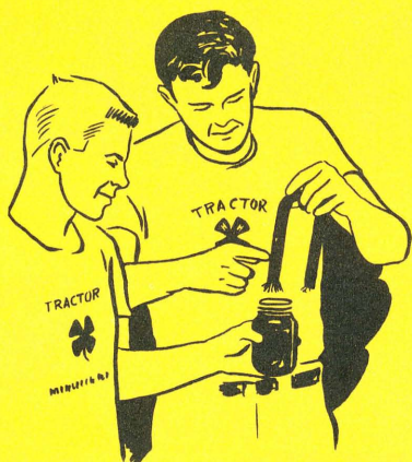
Fig. 20 Using a magnet is a good test for metal particles in your gear lubricant.
