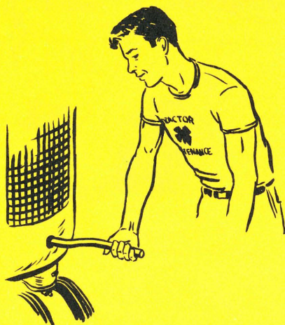
Fig. 3 Checking compression by cranking the engine.
