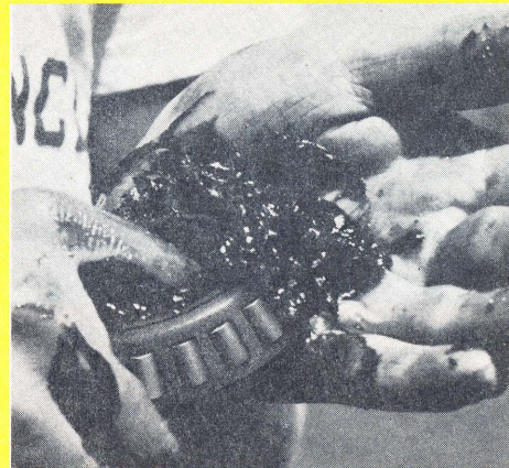
Fig. 16 How to pack a bearing.
