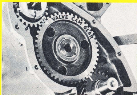
Fig. 2 Camshaft gear is twice the size of the driving gear at lower right. Note timing marks.
