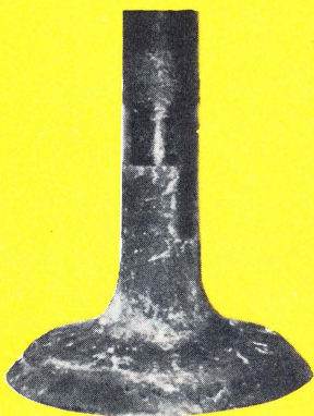
Fig. 4 A burned valve.
