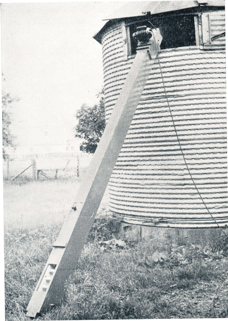
Fig. 36. The Michigan conveyor elevator for handling small grain, shown with hopper removed.
