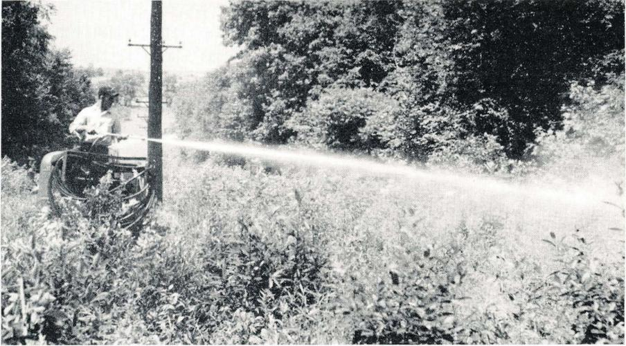
Fig. 3. Power sprayer and spray gun for use in brush control. High pressure aids in getting spray to penetrate mass of foliage. (Photo—Dow Chemical Company)
