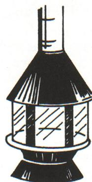
Fig. 6. A free-standing or prefabricated fireplace.
