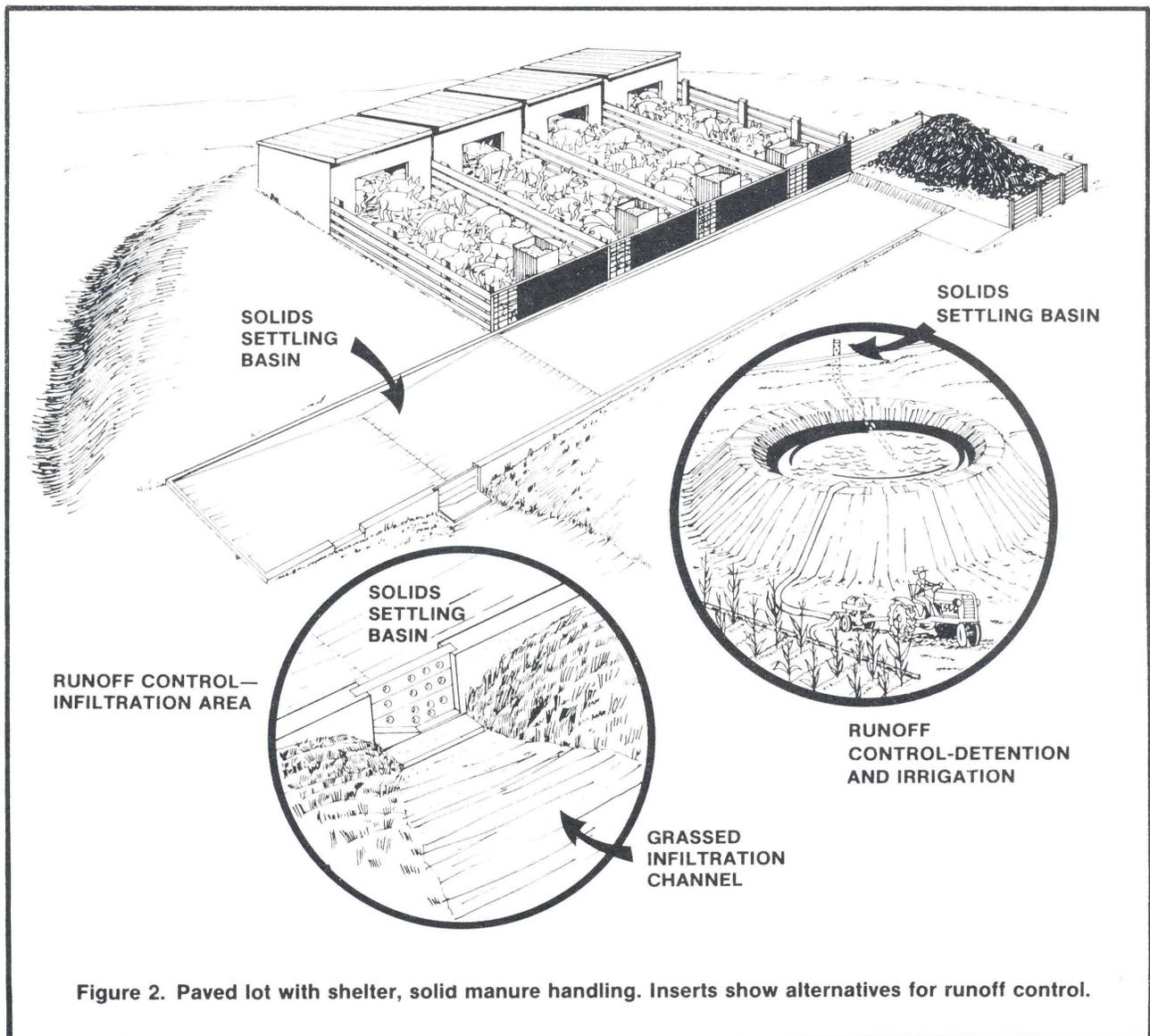
Figure 2. Paved lot with shelter, solid manure handling. Inserts show alternatives for runoff control.
