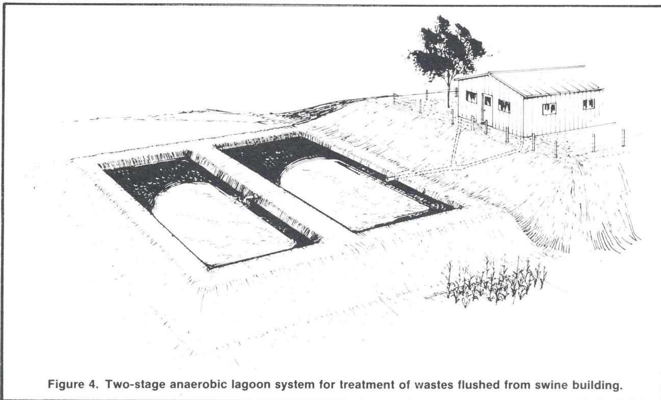
Figure 4. Two-stage anaerobic lagoon system for treatment of wastes flushed from swine building.
