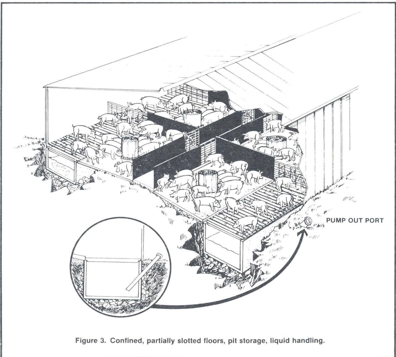
Figure 3. Confined, partially slotted floors, pit storage, liquid handling.
