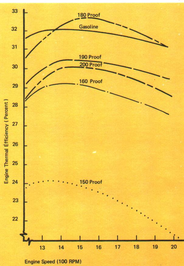
Figure 3—Effect of alcohol water content on engine thermal efficiency for alcohol used in a laboratory engine (5).
