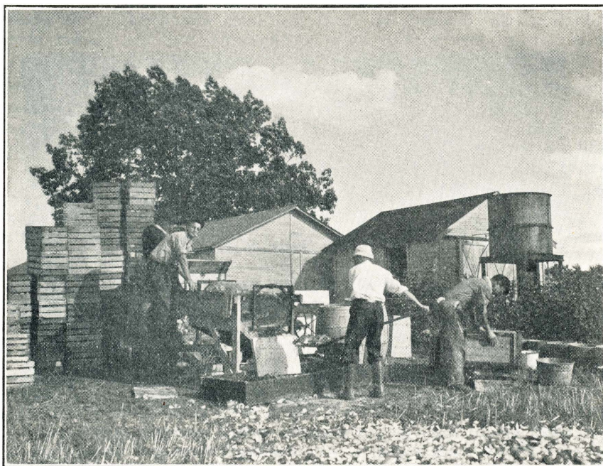
Fig. 10. Threshing cucumber seed. The hopper is equipped with corrugated rollers, which crush the fruits and the revolving wire mesh cylinder separates the seed and juice from the rinds. The storage tank in the rear supplies water for washing the seeds from the fermented pulp.
