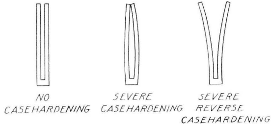
Fig. 22. Preparation of moisture content and casehardening samples: section to be room dried before conclusion is made as to casehardening.
