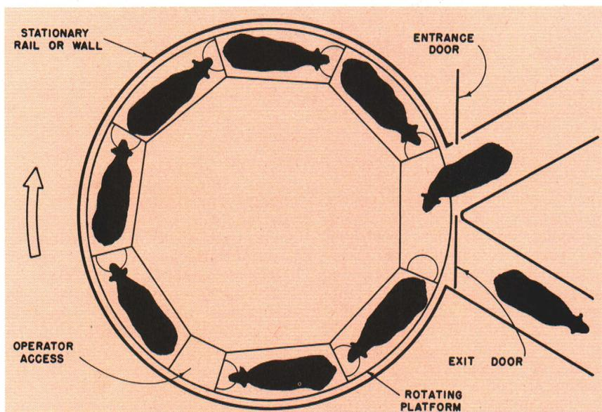
Figure 1—Rotary tandem
