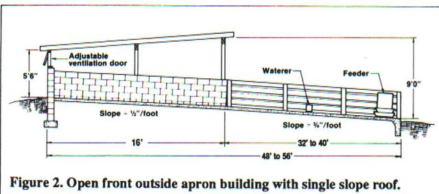
Figure 2. Open front outside apron building with single slope roof.
