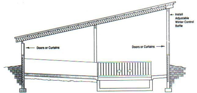
Figure 6. Single slope roof, partial slats building.
