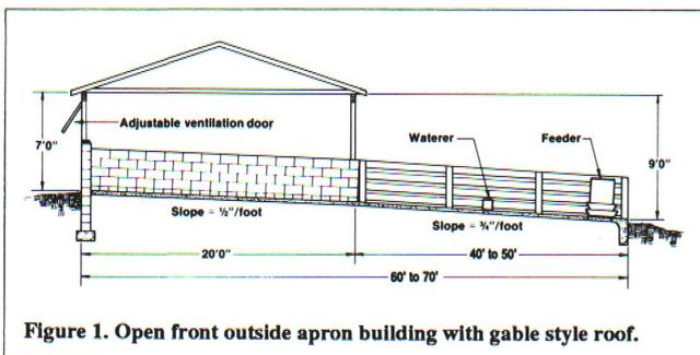
Figure 1. Open front outside apron building with gable style roof.
