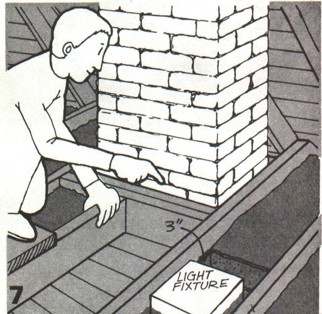
The space between the chimney and the wood framing should be filled with *non-combustible* material, preferably unfaced batts or blankets. Also, the National Electric Code requires that insulation be kept 3" away from light fixtures.
