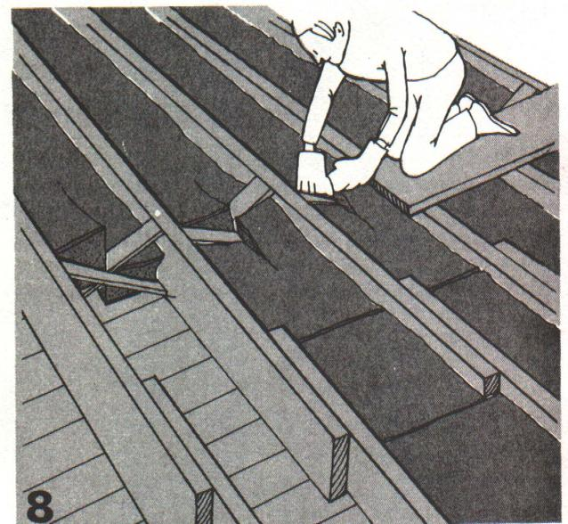
Cut ends of batts or blankets to fit snugly around cross bracing. Cut the next batt in a similar way to allow the ends to butt tightly together. If page 42 calls for an R-Value that requires a second layer, place it **at right angles** to the joists.
