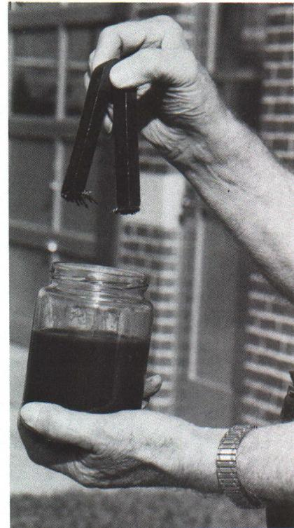
**Fig. 2 — There may be a serious problem if a magnet pulls metal chips and particles from a sample of transmission lubricant.**
