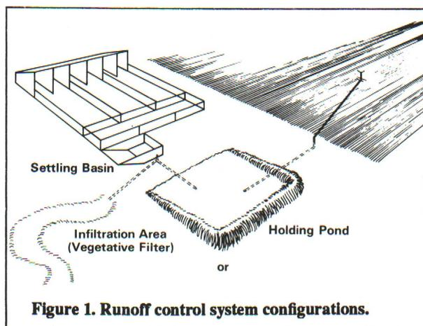
Figure 1. Runoff control system configurations.
