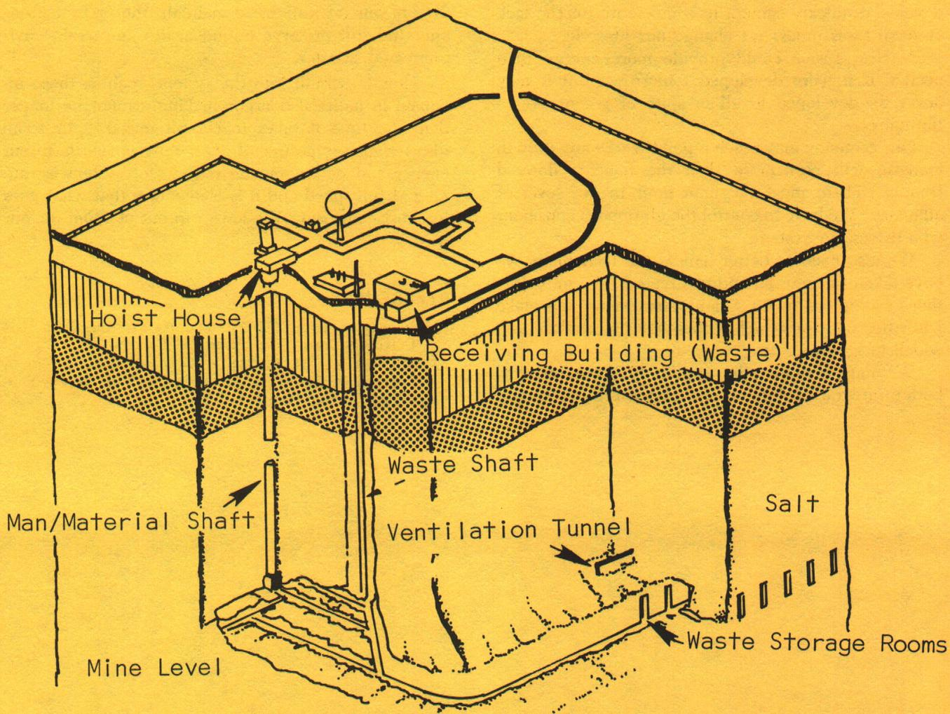
**Figure 1—Artist's conception of a bedded salt repository for solidified high-level radioactive wastes. The Storage area is 1,000 to 2,000 feet underground. (Photo courtesy Oak Ridge National Laboratory and U.S. Atomic Energy Commission.)**
