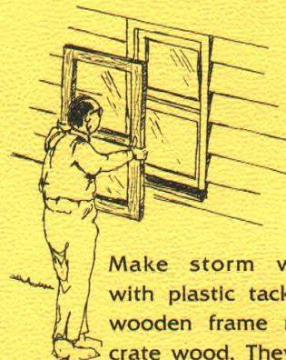
Make storm windows with plastic tacked to a wooden frame made of crate wood. They can be put outside or inside of windows.
