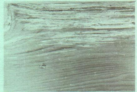
When the moisture content of wood is about 25-30% (possibly 20%, for some imported woods), spores germinate and form cell strands visible only by high magnification. These cells (*hyphae*) grow into and through wood.
