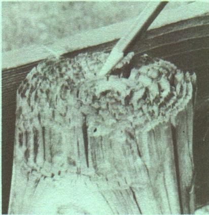
Fig. 9. Springwood portion of treated post eroded by soft rot.
