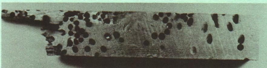
Fig. 18. Shipworm damaged wood cut from rafted logs.
