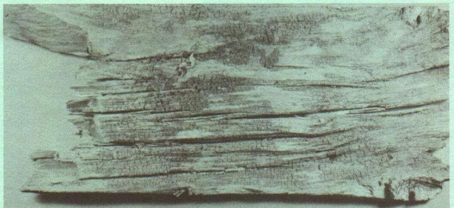
Fig. 8. Board surface destroyed by soft rot. Note small cross checks.
