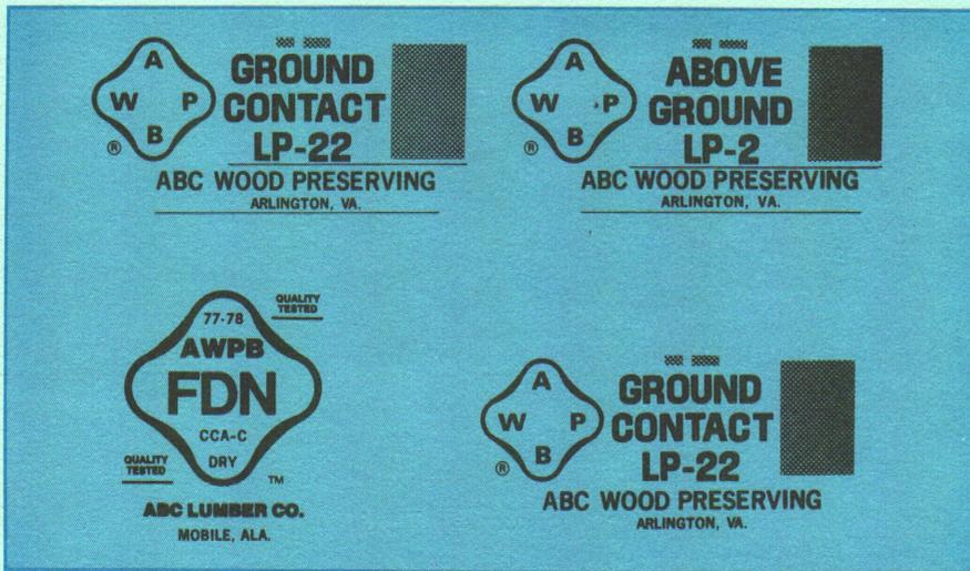
Fig. 3. Identification marks used on treated lumber.
