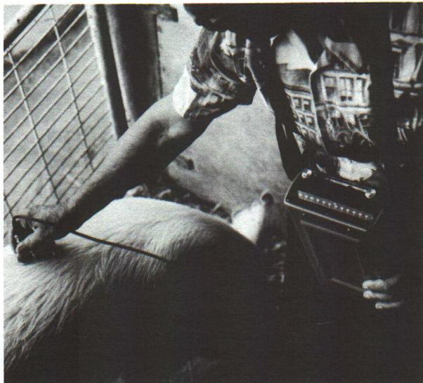
**Figure 4b. Ultrasonically measuring for backfat thickness.**
