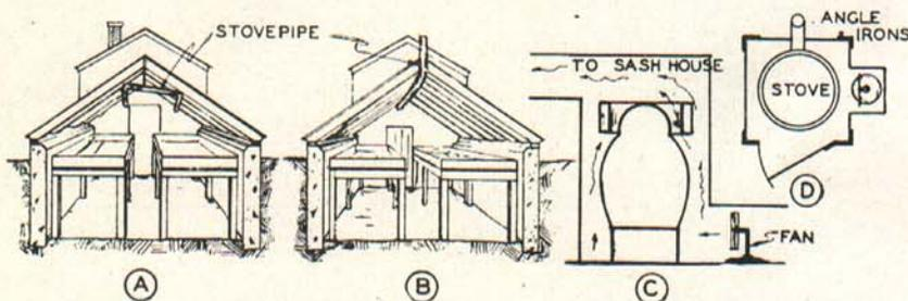
A building of this size can be heated conveniently with a stove or small furnace. The stove may be located in the head house and sometimes the smoke pipe is extended through the sash house just below the sash as shown at A and B in the above drawing. In using this method of heating, precautions should be taken to prevent leakage of smoke into the house. Stove pipe made in six- or eight-foot lengths and the joints soldered is sometimes used.
