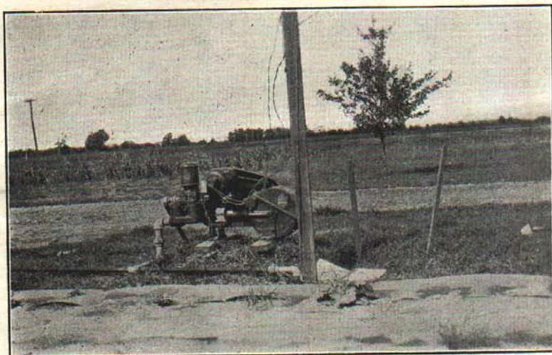
Fig. 15.—A piston pump operated with an electric motor pumping from 4 shallow wells.
