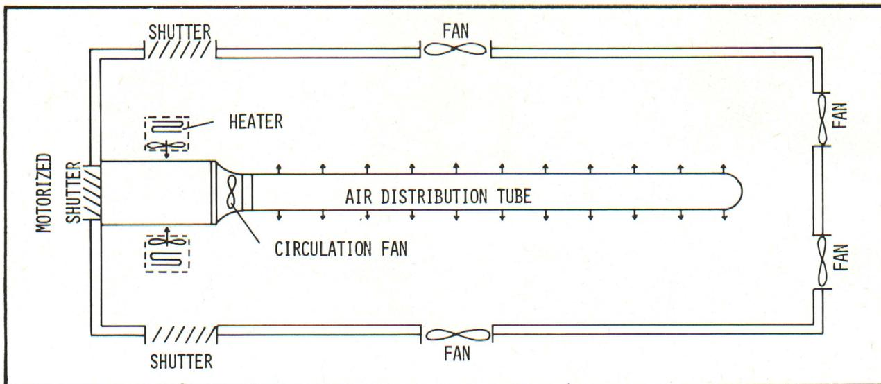
Figure 4. Positive pressure intake and air distribution.
