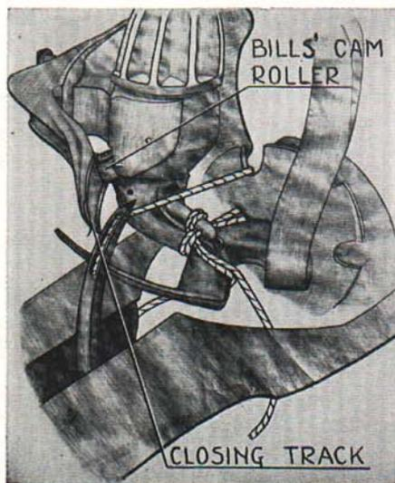
Fig. 10. Step 5 in the Tying Process.
