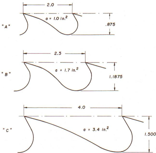
Fig. 6—Gullet space and tooth dimensions of selected band saws "A", "B", and "C".
