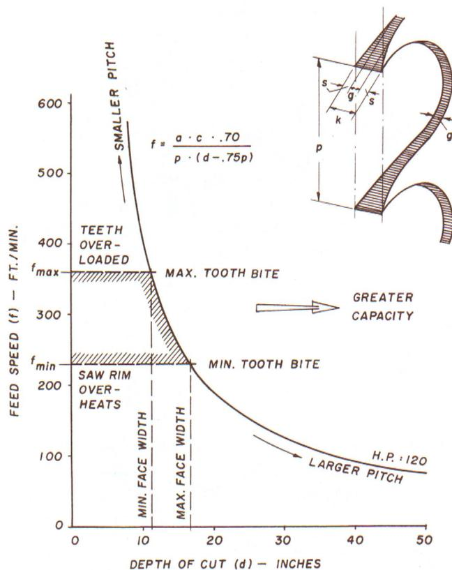
Fig. 3—Operating characteristic of band saw "A".
