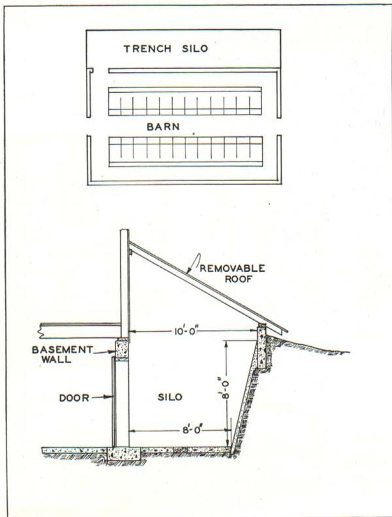
Fig. 5. A convenient location for a trench silo.
