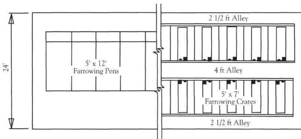
**Figure 2. Arrangement of two rows of crates or a single row of pens in a 24-foot wide building.**
