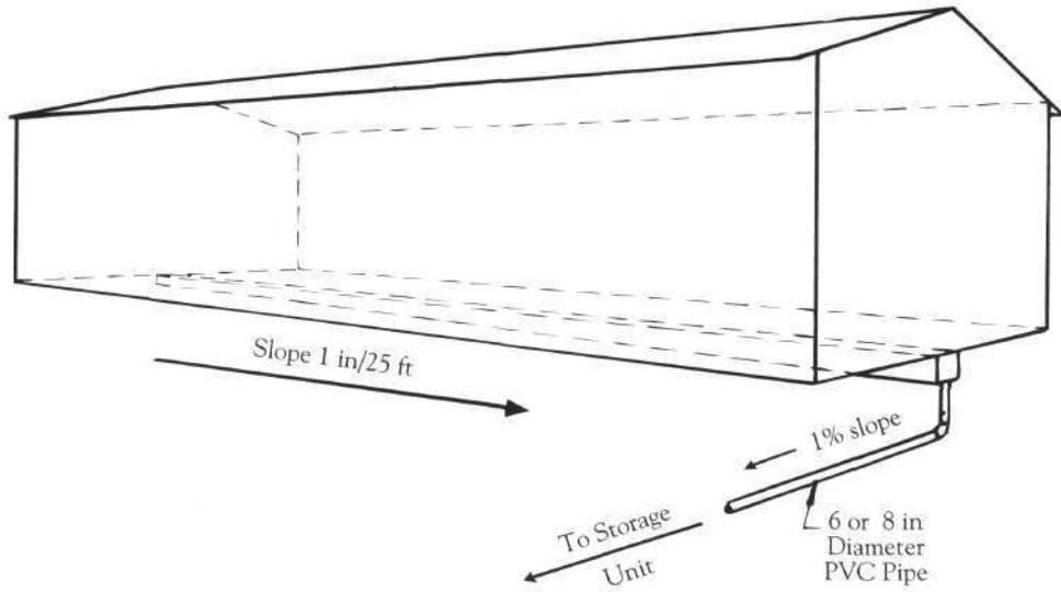
Figure 9. Slope of gutters in a gravity drain system.
