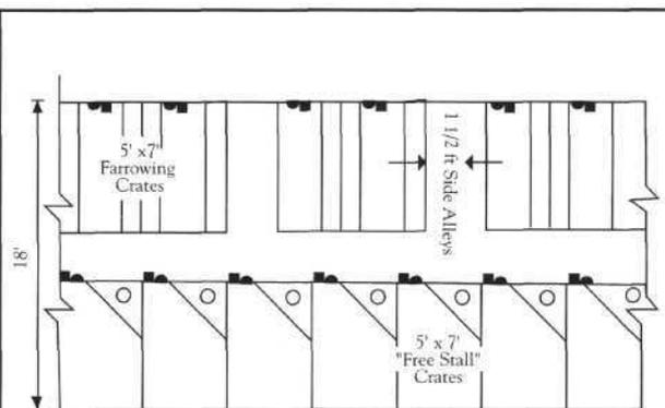
**Figure 3. Arrangement of crates and "free stall" crates in an 18-foot wide building.**
