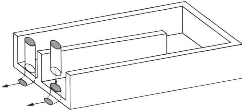
Figure 10. "Hairpin" gravity drain gutter.
