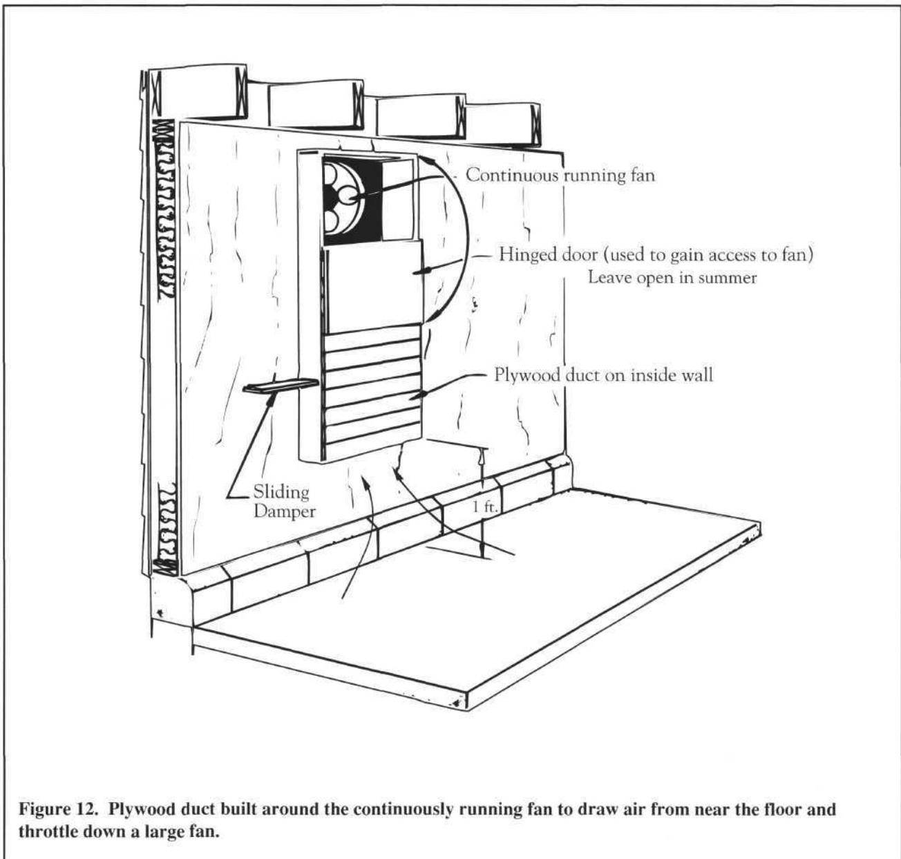
Figure 12. Plywood duct built around the continuously running fan to draw air from near the floor and throttle down a large fan.
