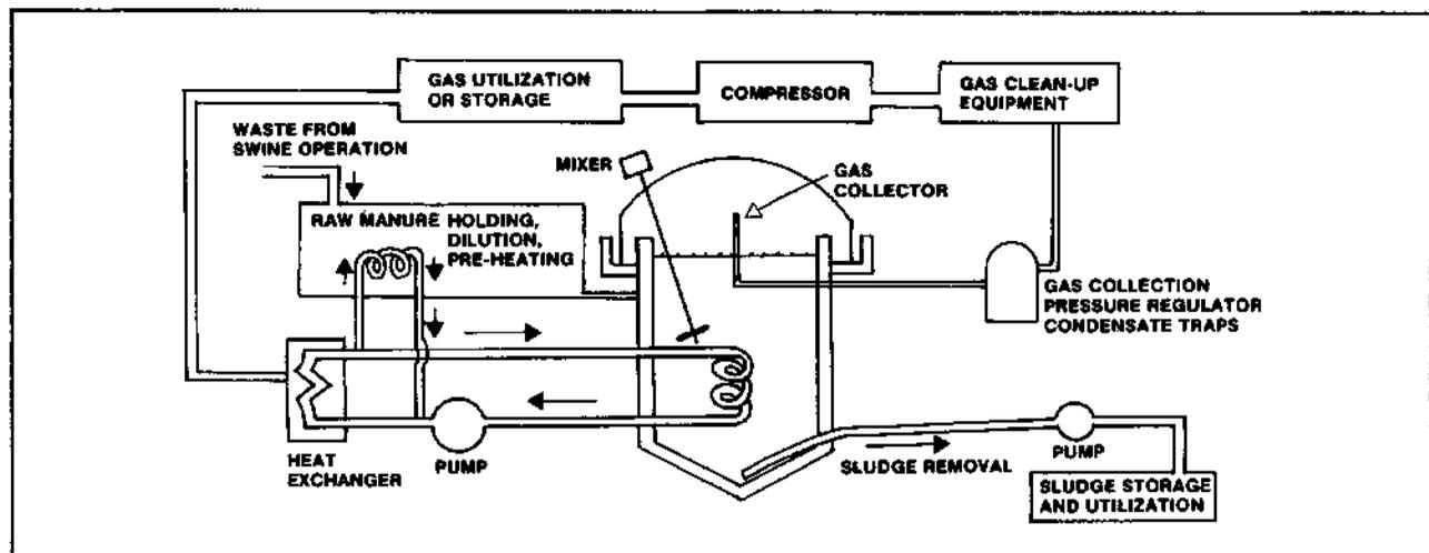
Figure 1. Anaerobic digester.
