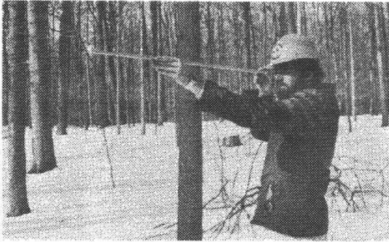
Fig. 4. To estimate basal area using an angle gauge, the observer turns a complete circle over the sampling point and counts the total number of trees larger than the width of the block.
