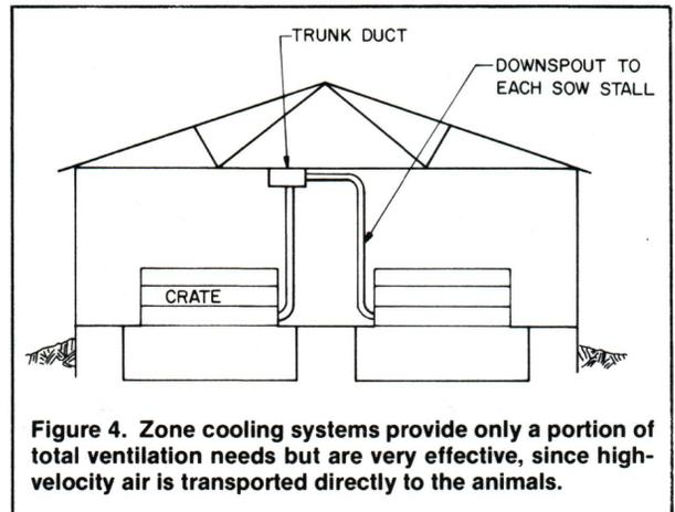
**Figure 4. Zone cooling systems provide only a portion of total ventilation needs but are very effective, since high-velocity air is transported directly to the animals.**
