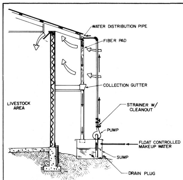
**Figure 3. In a sidewall mounted evaporative cooling system, ventilation exhaust fans pull hot outside air through wet fiber pads. Heat from the air is used to evaporate the water, thus lowering temperatures but increasing the relative humidity. Consider modifying the baffle for down-the-wall air flow for maximum benefit when the cooling system is in operation.**
