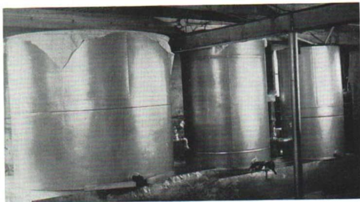
Fig. 29. Honey storage and settling tanks, below extractors.
