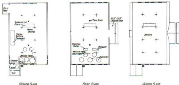
Fig. 35. Floor plan for 36' x 60' Gothic type honey house.
