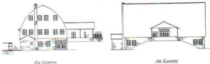
Fig. 31. Gothic type honey house. Note that two loading levels are available.
