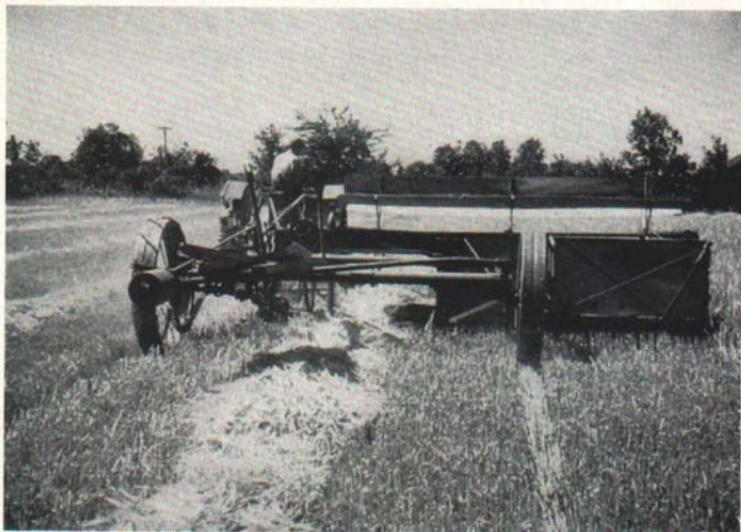
*Fig. 3. Cutting and windrowing barley with a windrowing machine.*
