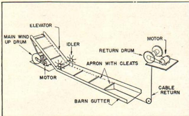
Fig. 1. Diagrammatic view of a "wind-up" type barn cleaner. Angle of elevator rise should not exceed  $30^{\circ}$ .
