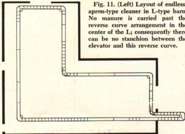
Fig. 11. (Left) Layout of endless-apron-type cleaner in L-type barn. No manure is carried past the reverse curve arrangement in the center of the L; consequently there can be no stanchion between the elevator and this reverse curve.
