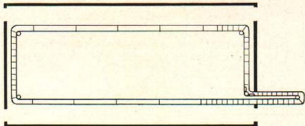
Fig. 10. (Above) Layout of endless-apron-type cleaner in two-gutter barn. Power unit is located on top of elevator (see Fig. 18). For details of reverse curve, see Fig. 19.
