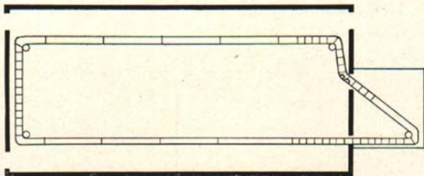
Fig. 9. (Above) Layout of endless-apron-type cleaner where land slopes away from end of the barn, permitting a manure spreader to drive under the extended gutter. This is all in one plane and no elevator is needed.
