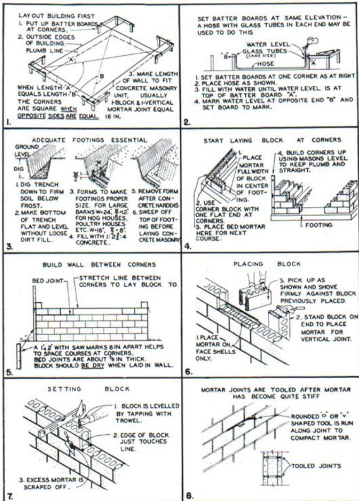
Fig. 5. Details of masonry wall construction.
