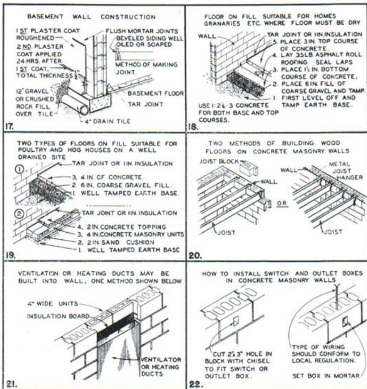
Fig. 5. Details of masonry wall construction—(Concluded).
