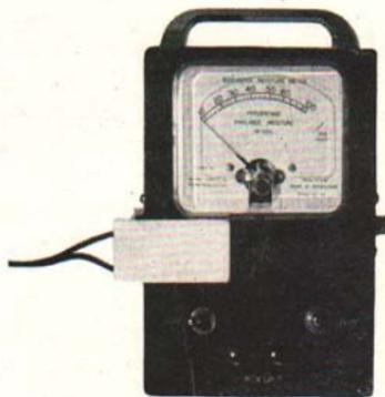
Fig. 2. Bouyoucos soil-moisture meter with plaster-of-paris block.
