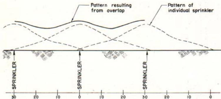
Fig. 7. Distribution of water from overlapping sprinklers.
