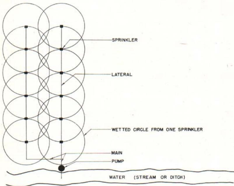
Fig. 4. Field layout for a portable system.
