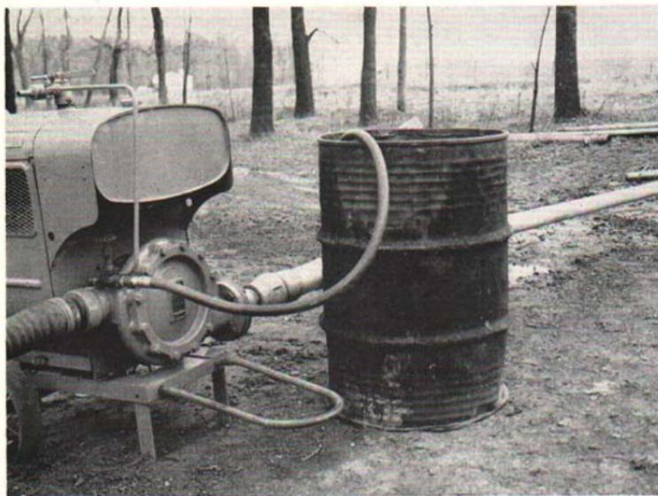
Fig. 1. Centrifugal pump drawing fertilizer solution from a drum, for application to a field through the irrigation water.
