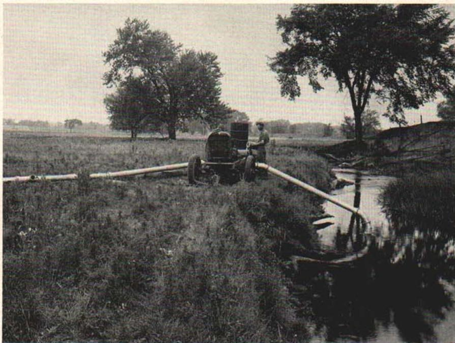
Fig. 2. For an efficient operation, irrigators depending on streams for their water supply must base plans on the flow "during the driest time of the driest years." The mobile unit pictured can pump 30,000 gallons an hour.
