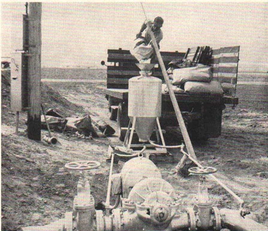
Fig. 6. One type of commercial fertilizer applicator which utilizes a pressure difference at a pump for feeding the solution into the sprinkler system.
