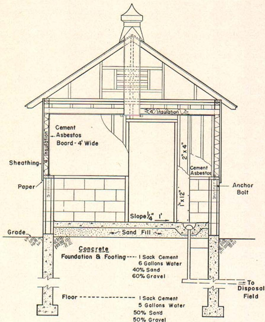
Fig. 5. Cross section of a typical frame milkhouse.
