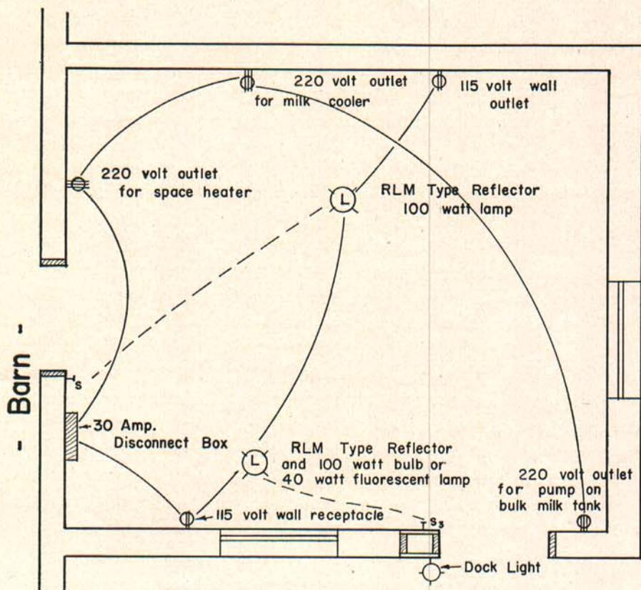
Fig. 8. Suggested wiring diagram for a farm milkhouse.
