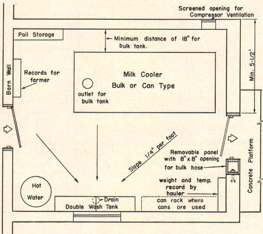
Fig. 2. Suggested layout for milkhous with doors on opposite sides. (See Table 1 for dimensions.)
