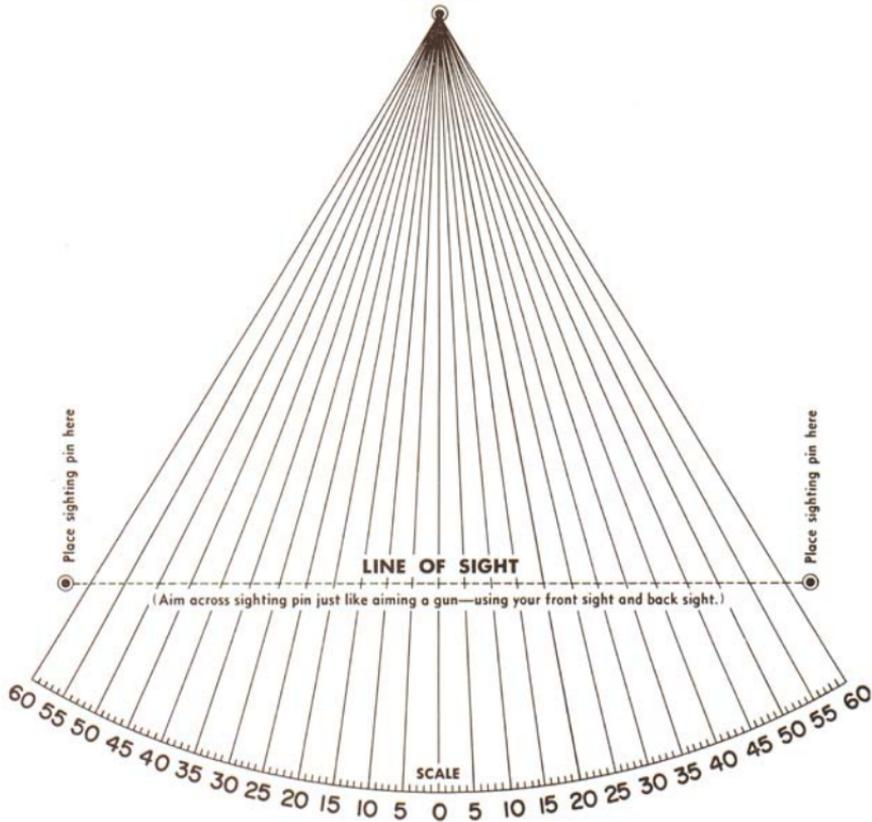
Read percent of slope directly on this scale. At this point where string rests on scale, the number indicates percent of slope, or the number of feet of rise or fall in 100 feet.
